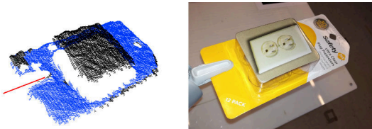
Fig. 2: An example of sliding area, considering the object shown on the right. The red line segment indicates the current grasp as the position and orientation of the gripper’s finger. The blue area shows the portion of the object’s surface on which the fingertip is allowed to slide.
