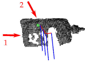
Fig. 9: The proposed in-hand path. Since a direct pushing from initial to goal contact point is not considered valid, the in-hand path uses two separate pushing directions.
