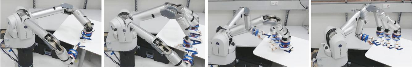
Figure 8. Real executions of the proposed planner using a WAM arm installed with a Yale T42 hand. The objects are perceived using a Kinect sensor installed over the tabletop. The plastic “Y”, “A”, “L” and “E” letters are grasped after executing the pre-grasp top-sliding manipulations planned by our planner. More example executions can be found in the supplementary video.
